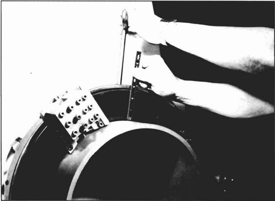
Photo 2: Centering clamshell with six inch (6") scale at each locator pad position.
