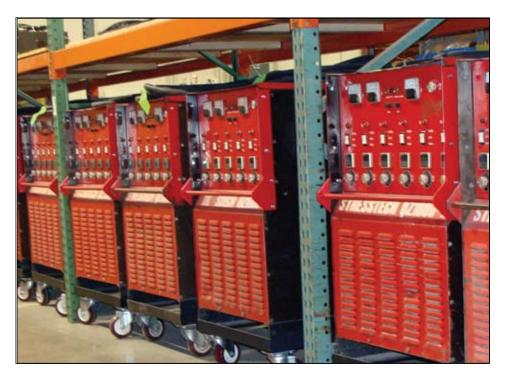
Operators only need to enter the "SOAK" temperature and the controller will automatically ramp from current temperature to setpoint at the specified ramp rate. The controllers can also be operated manually by disabling the ramping function and using the percentage timer.
