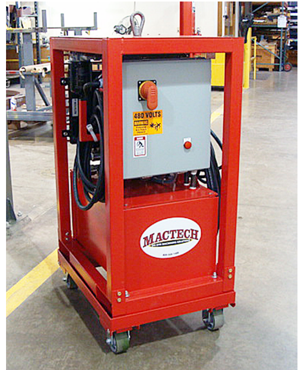
Figure 1-2 – Hydraulic Power Unit
