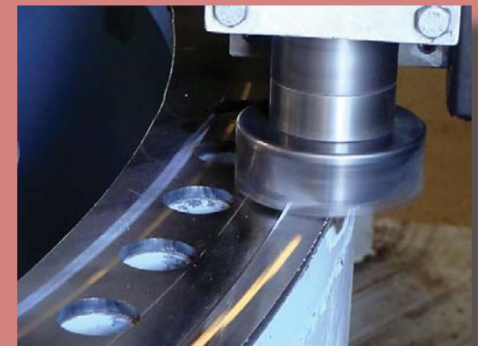
Wind Turbine Base Flange Facing
