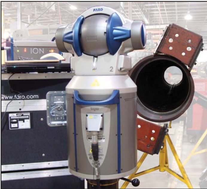
Laser Tracker Bore Inspection
