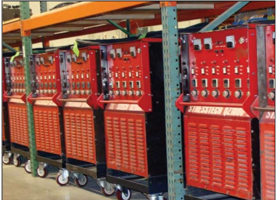
Operators only need to enter the "SOAK" temperature and the controller will automatically ramp from current temperature to setpoint at the specified ramp rate. The controllers can also be operated manually by disabling the ramping function and using the percentage timer.
