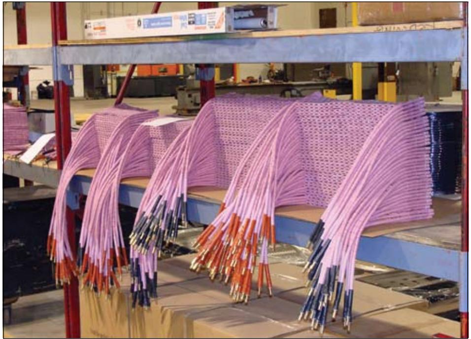
**STRESSFLEX Pads** are equally rated 50 AMPS at 80 Volts and are available in many stocked sizes and can be custom built for specialty jobs. Our stocked sizes will preheat or stress relieve almost any job imaginable. They are used in refineries, power plants, construction, and fabrication applications, just to name a few. They can be used in any combination while maintaining the same watts per square inch of power.
